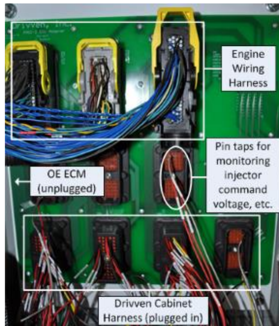
Figure 6.5 Engine harness, Drivven harness, and OE ECM harness adapter board
