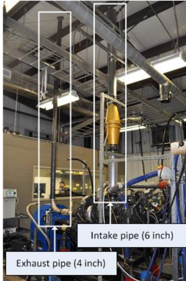
Figure 6.6 Intake and exhaust plumbing with vertical orientation
