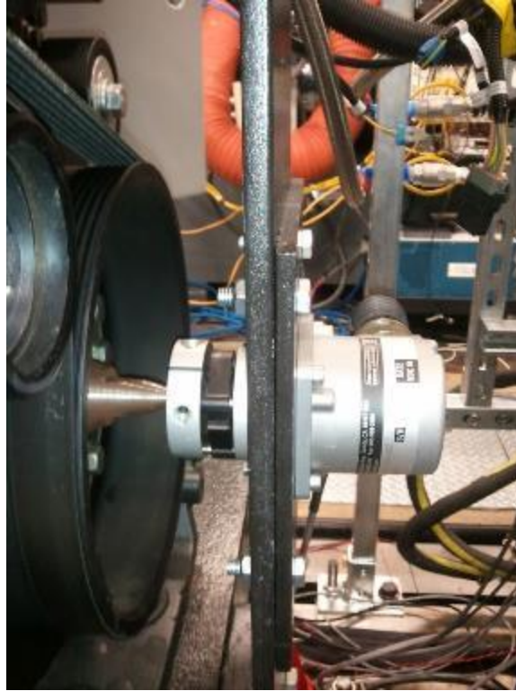
Figure 6.14 Encoder bracket, crankshaft adapter, and coupler
